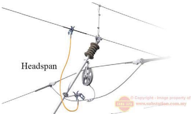
Headspan using Single Short Rail Earth
