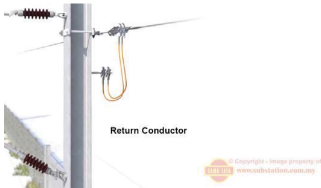
Return Conductor using Double Short Rail Earth
