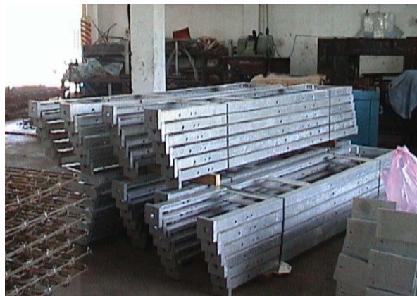
Circuit Breaker steel support structure
