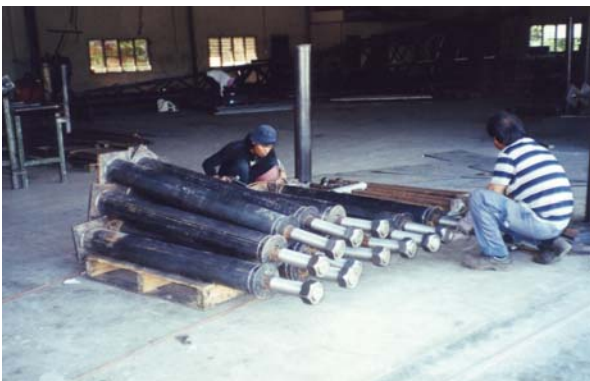
Anchor Bolts with Sleeves and Embedded Plate
