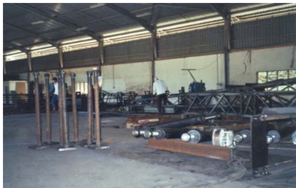
Anchor Bolts with Foundation Embedded Plate
