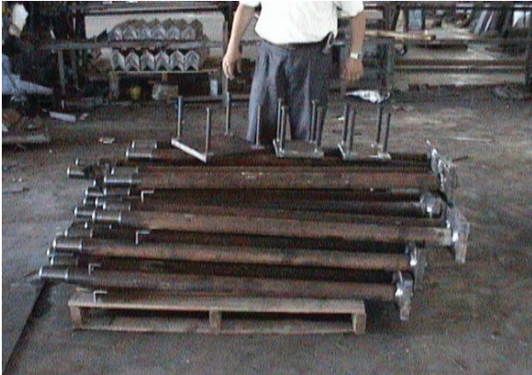
Anchor Bolts with Foundation Embedded Plate
