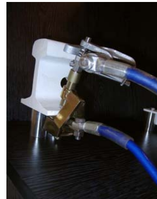
Interlocked clamps being applied to Flat bottom Rail Section
