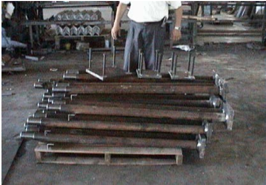
Anchor Bolts with Foundation Embedded Plate
