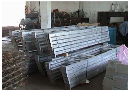
Circuit Breaker steel support structure
