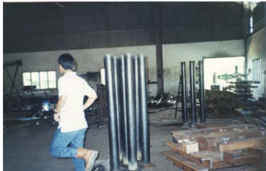
Anchor bolts with welded plates
