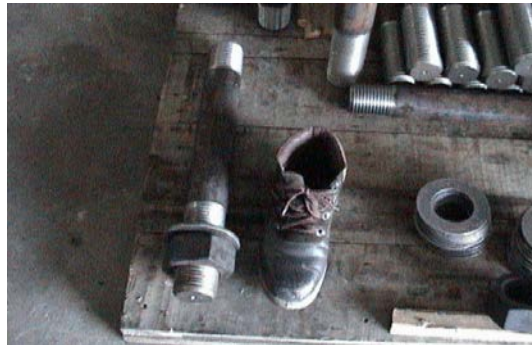
Anchor Bolts for Turbines
