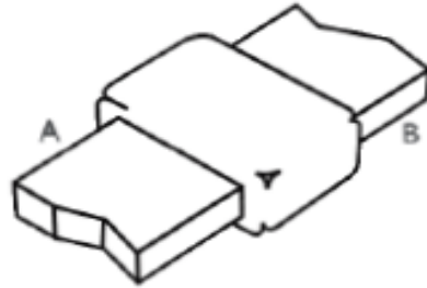
Horizontal flat bus bar end to end
