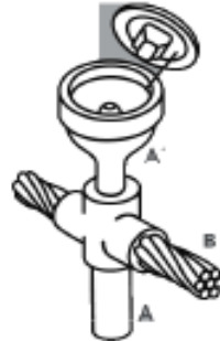
Horizontal cable thru and ground receptacle to the top of ground rod
