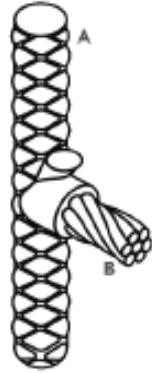
Horizontal cable tap to vertical rebar
